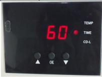
Press button after temperature setting and the time light is on. Using the arrows select the time according to different transfer material.
