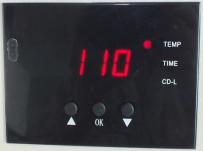
Press button, the temp light is on. Using the arrows select the temperature, according to different transfer material (Normally 180°C~200°C)
