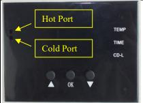
Note: There are two small ports in the front side of the digital display. If the real temperature is lower than digital controller shown, you can adjust the "hot port"; Clockwise to Raise the temperature; anticlockwise to reduce the temperature.
