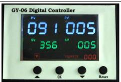
Press M button to operating mode. Counter is "transfer cycle", from 0~999 Sec. Press "Reset" for 5 seconds to return the counter to "0".
