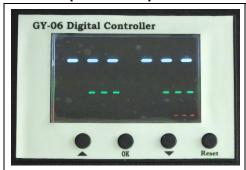
Turn on power switch, temperature light is ON. The digital display shows as above.
