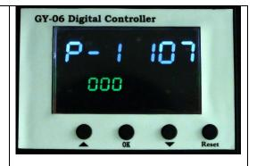
When SV and PV has a big difference, press button for 5 seconds, and press button again to adjust the temperature. If SV&PV has difference of 20 degrees, Press arrows "△" or "▽" to set to 20.
