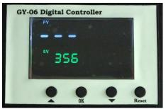
Press button, the temp light is on. Select with arrows the temperature according to different transfer material (Normally 180°C~200°C)
