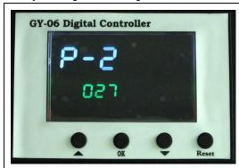
When SV and PV values show a big difference, press button for 5 seconds, and press button again to adjust the temperature.
