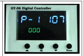
When the temperature shown on the display is not the same as the actual temperature on the heat platen, press button for 5 seconds to reset mode:
