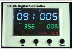
Press button to enter operating mode. The counter denotes the number of "transfer cycles", with a range of 0~999. To reset the counter to "0" press "Reset" for 5 seconds".
